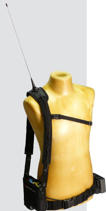
RPU 300-xx (main transmitter section) complies with ETSI specs: ETS 300 454.
